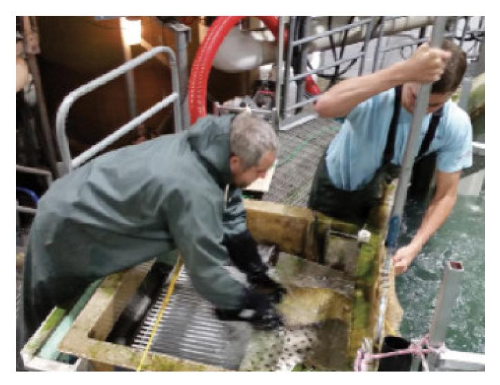
In testing, sliding the fish by hand into the outlet channel allowed manual orientation of the salmon to test fish transfer through the system.
