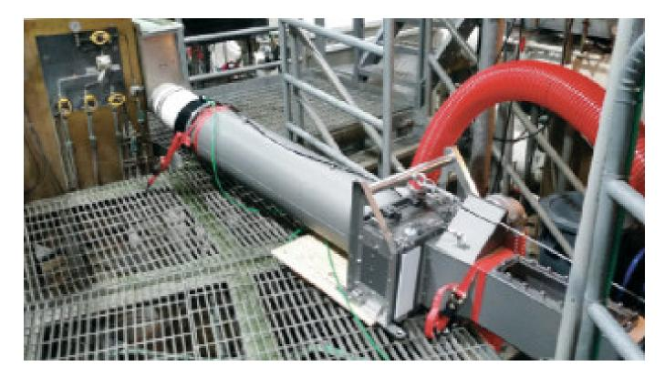
The "accelerator" is attached to the side wall drop box of a tank (left rear). Fish that enter the system are "whooshed" along via the exit at the lower right. The red tube pulls air out of the system. A second tube underneath (not shown) pushes air.
