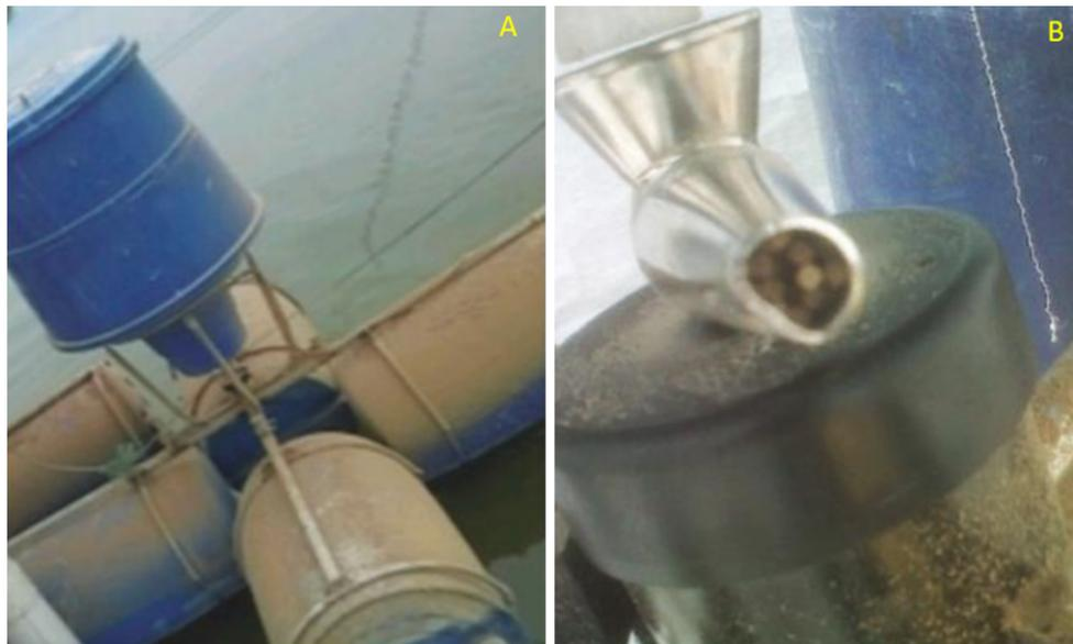
Fig. 3: Fine accumulations in the floating tanks of an automatic feeding system (A); feed blockage in a type V dispenser – note the amount of fines generated around it (B).
