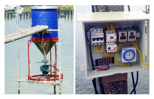
In small culture ponds, an automatic feeder can broadcast feed in a radius of 10 m and feed 600,000 shrimp. Timers control the broadcasting times and intervals of feeding.
