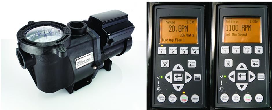
Programmable variable-speed pumps can provide a constant flow to an aquaculture system even when pressures vary within the system. “Backpack” controller systems can display motor speed or pumping flow rate.
