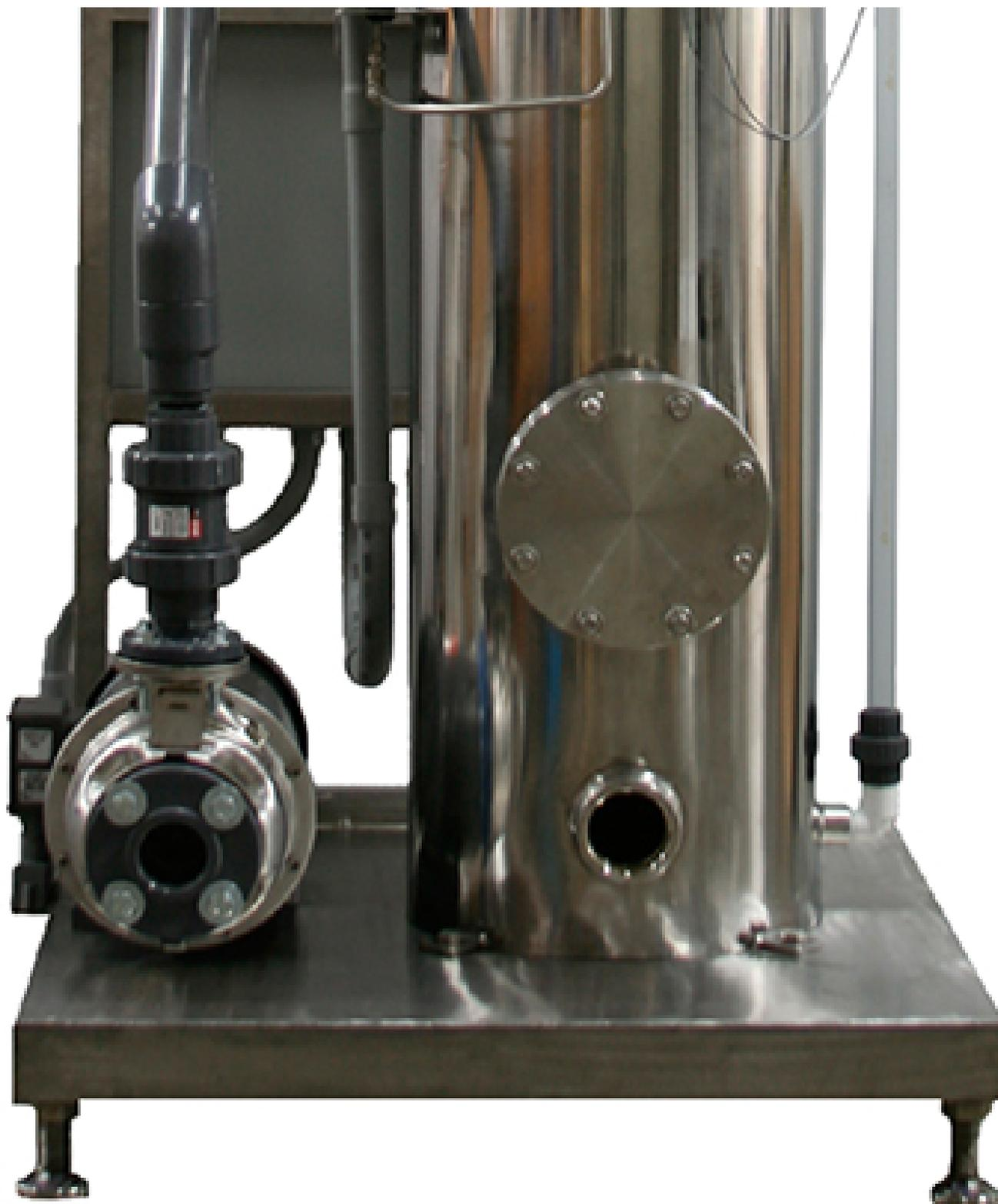
Fig. 1: Pressurized packed column oxygenators can be combined with constant flow pumps and programmable controls to provide efficient oxygen addition to a wide variety of aquaculture systems.
