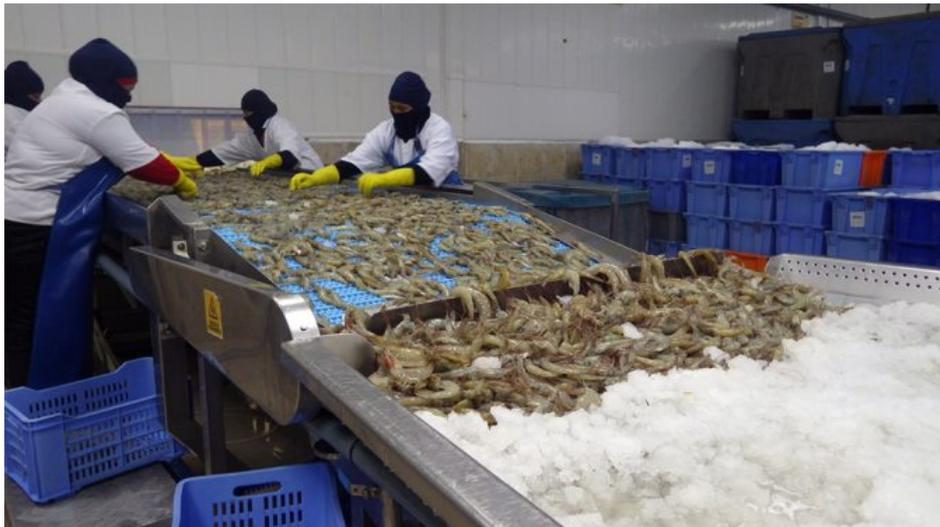
View of a well-organized and efficient initial inspection and washing tank station.
