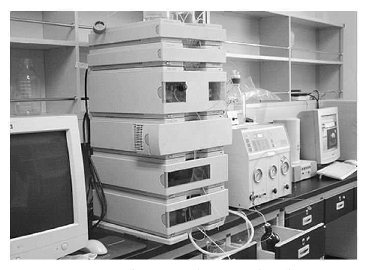
Liquid chromatographers are used for separation, identification, and quantification of high boiling point, poor heat stability, or large molecules.
