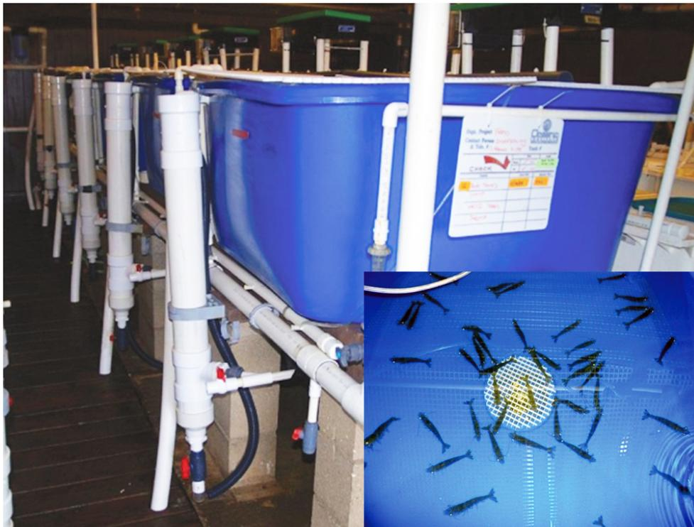
The experiment was conducted in an indoor flow-through water system with a series of 550-L polyethylene tanks.
