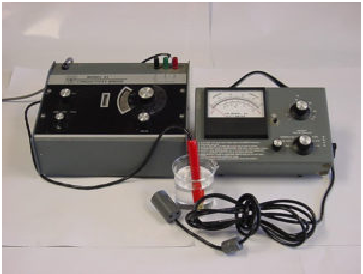
Fig. 1: A laboratory bench conductivity meter (left) and a portable conductivity meter (right).
