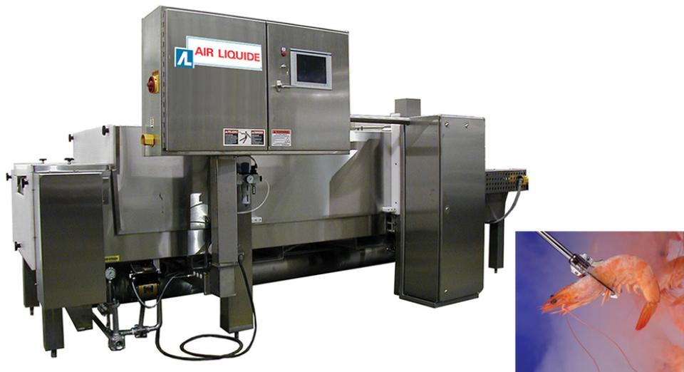
Liquid nitrogen freezing equipment can form a crust on shrimp in a few tenths of a second. This freezer is designed for use in association with a mechanical deep freezer.
