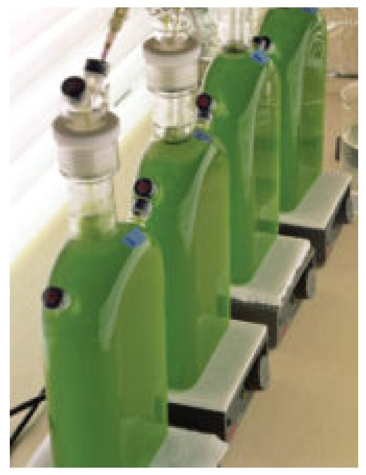
Photobioreactors like these lab-scale units are self-contained systems that continuously pump water containing algae through clear vessels of various types to expose the algae to light for growth. (Photo courtesy of the U.S. Department of Energy National Renewable Energy Laboratory.)
