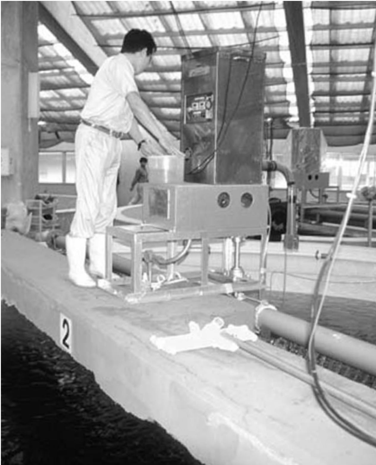
The automatic feeder in this indoor recirculating system feeds flounder in a Japanese operation.
