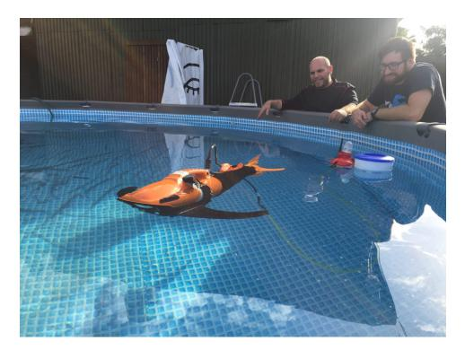
Aguaai's robotic fish "Nammu" mimics how actual fish swim. The ability of the robot to swim alongside fish and be accepted by them allows for superior data acquisition. Photo courtesy of Aquaai.
