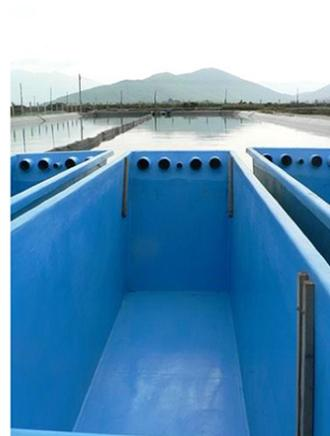
The fiberglass raceways can be suspended on simple pontoons in new or existing farm ponds to nurse groupers, barramundi, tilapia, and cobia.
