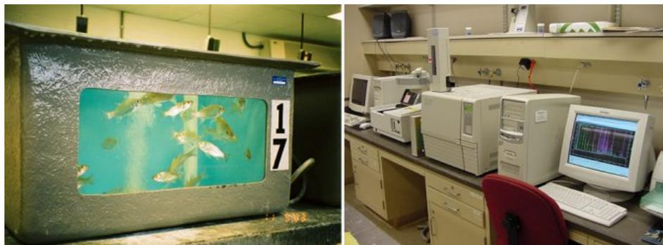
Some of the fish used in the study (left), and gas chromatography equipment used to determine fatty acid composition of HSB fillets (right).
