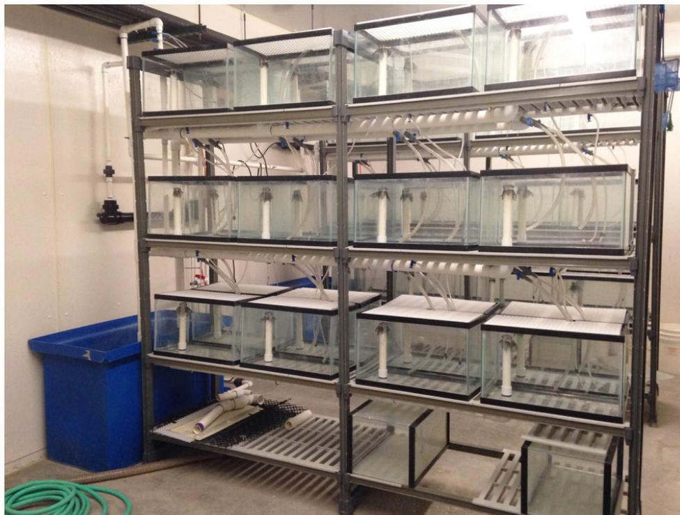
Fig. 4: One of three APL-WCAC bank systems with 37-liter aquaria and a recirculating system.
