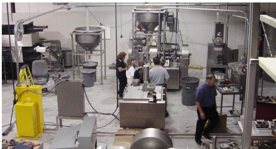
Properly proportioned ingredients, together with adequate mixing time, ensure the production of formula that meets the standards for the species and growth stage for which it was designed.
