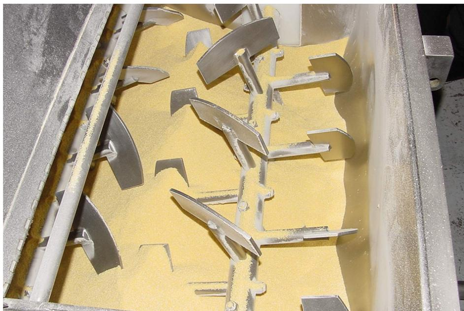
Regular examination of mixer components for wear and material build-up helps ensure clean, consistent operation.
