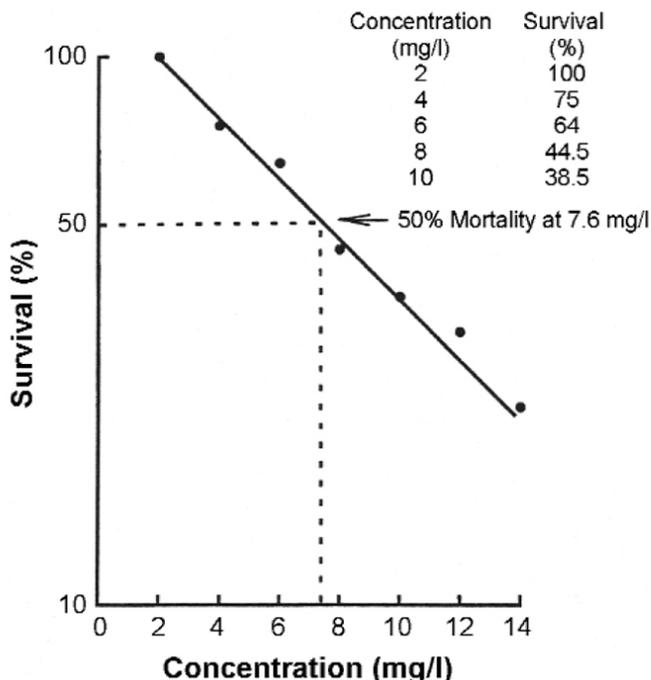
Fig. 3: Graphical estimation of LC<sub>50</sub>.
