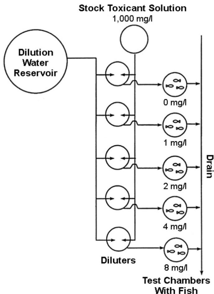
Fig. 2: Example of a flow-through toxicity test.
