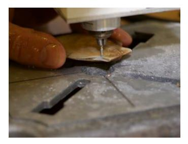
Without automation, using specialized equipment developed in Japan, scallop farmers using the earhanging technique have to drill the oysters individually, by hand.
