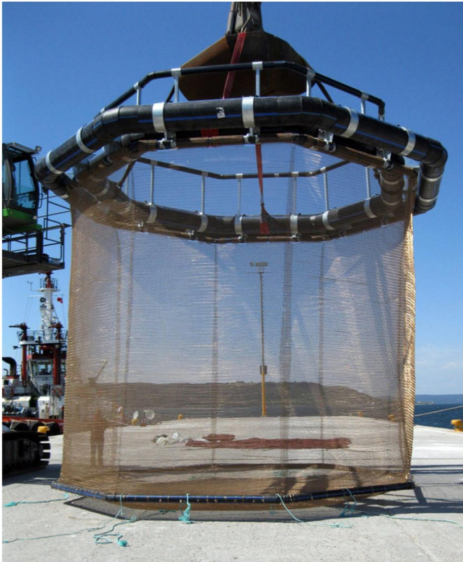
Testing has shown that copper net chambers retained their shape better than similar-sized nylon net pens.
