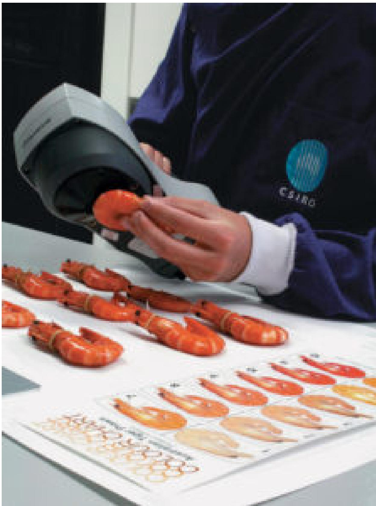
Quantitative measurements of shrimp color are possible using modern hand-held colorimeters.
