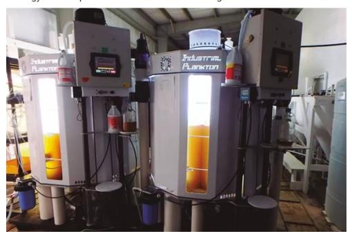
An example of the use of photo-bioreactors in a commercial laboratory producing oyster larvae in Nova Scotia, Canada.
