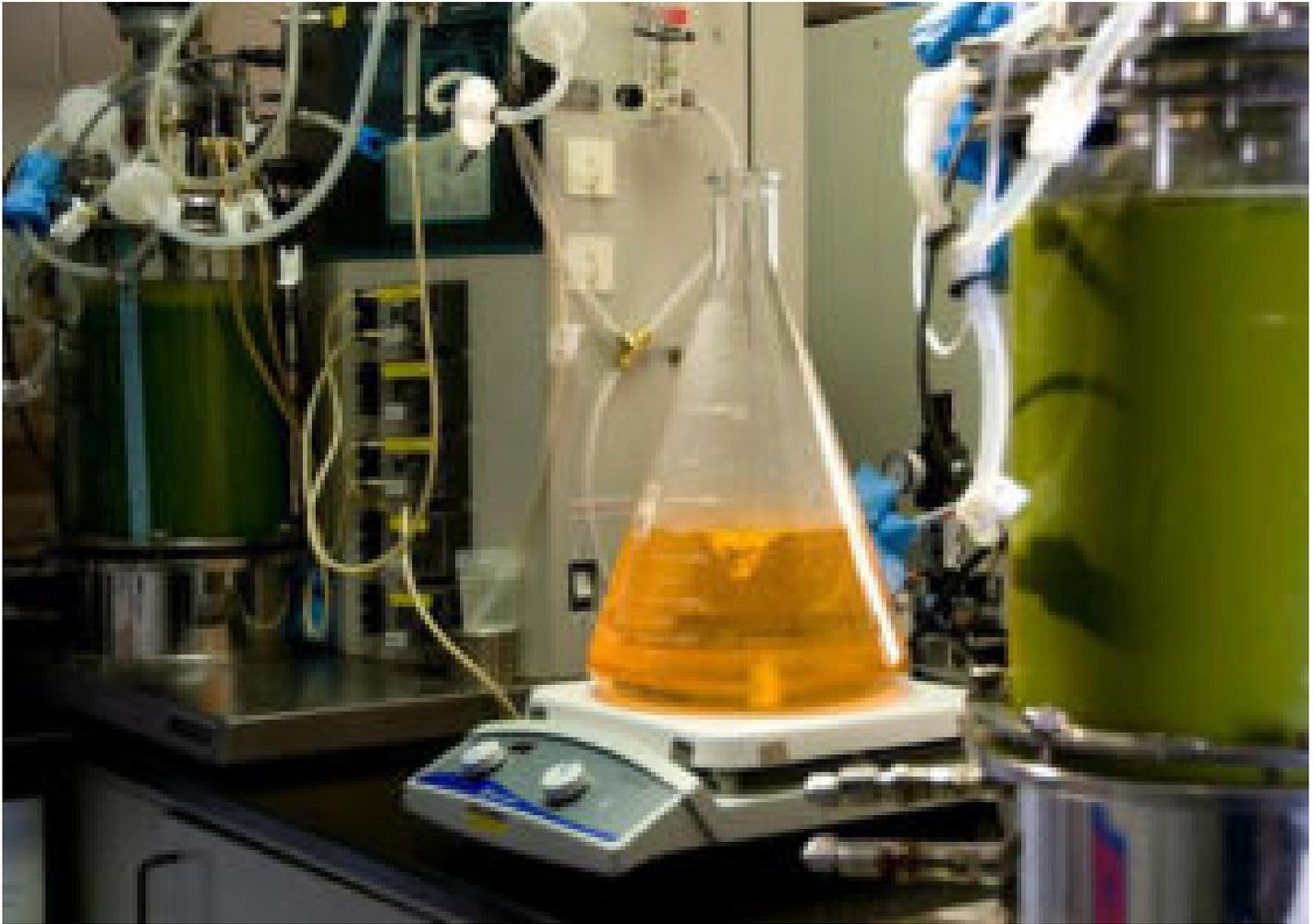
Research into the varied applications of algae is assisted by the use of 5-L fermentation vessels such as those pictured above. These vessels allow algae to be produced by a feed batch technique that results in unique nutritional properties.
