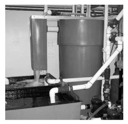
Fluidized-bed biofilter in operation. Photo courtesy of Aquaneering Inc.
