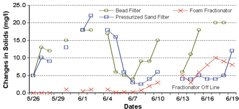
Fig. 1: Changes in settleable solids in raceways operated with bead filter, pressurized sand filter, and foam fractionator over 74-day nursery trial.
