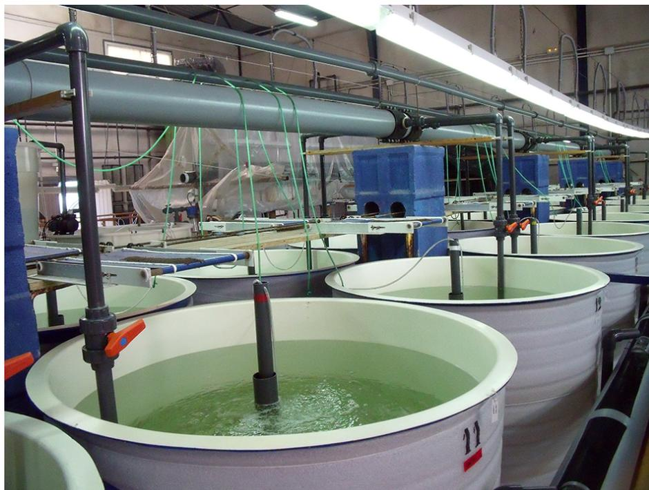
The recirculating system used in the trial had a biofiltration unit, sand filter and protein skimmer.
