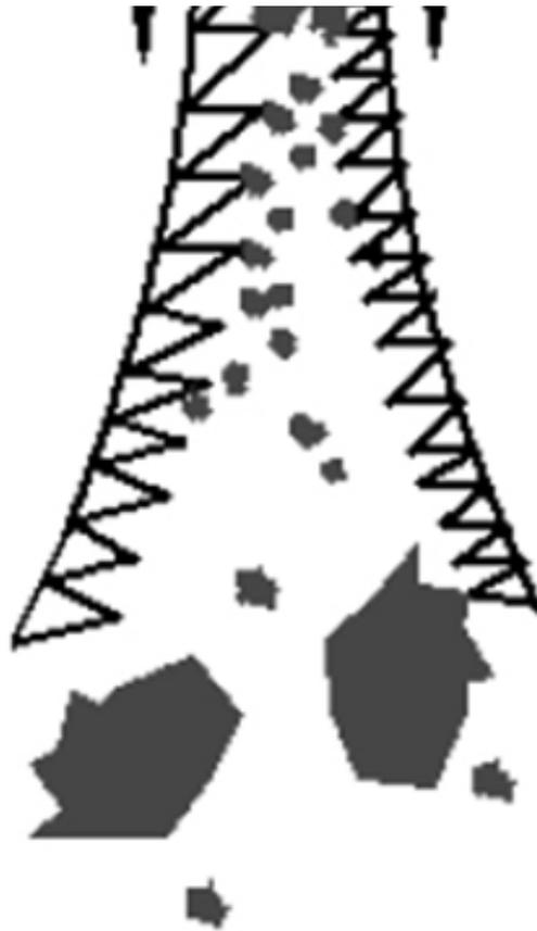
Fig. 2: Crumbler rollers rotate at different speeds and have different corrugations.
