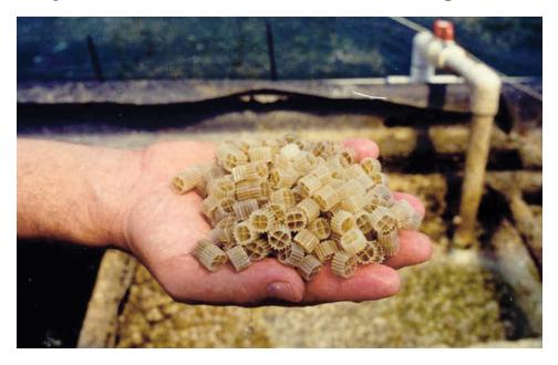
Biofilms can be beneficial too: Many recycling systems use specially designed media to increase the surface area available for adhesion of biofilms rich in nitrifying bacteria.
