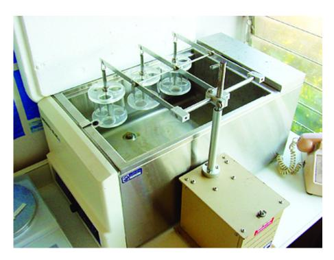
Fig. 3: Water stability testers immerse and agitate feed samples.
