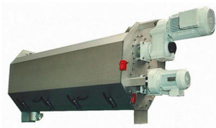
Many pre-conditioners have high radial mixing in a chamber where steam and water are injected. In a second chamber, more axial mixing occurs and the ingredient meal is hydrated there. Images courtesy of Buhler.
