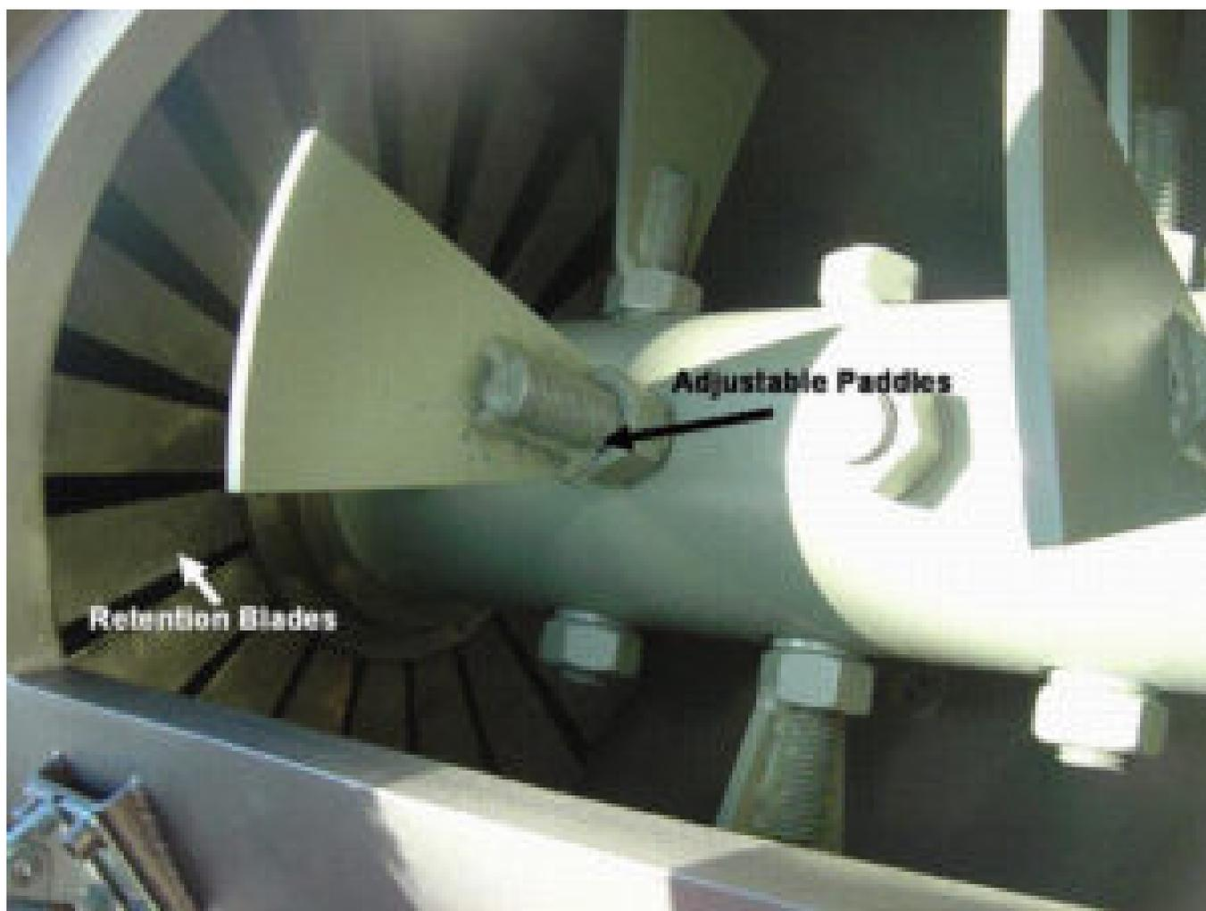
Paddles in most preconditioner can be adjusted by the operator to achieve the best configuration.
