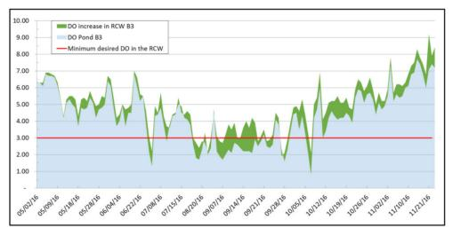
Fig. 4: Illustration of the early morning dissolved oxygen concentration in the pond (blue area) and inside the raceway (green area) in pond B3. The green area above the blue area indicates how much oxygen the aeration device added to the water at the entrance of the raceway, keeping dissolved oxygen levels inside the raceway often above 3 mg/L (minimum desired level) and seldom below 2 mg/L, even when pond D0 approached values close to 1 mg/L.
