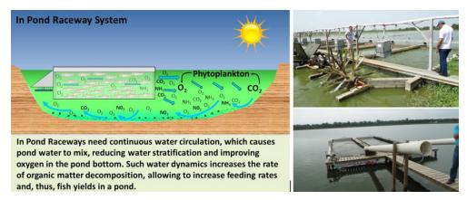
Fig. 1: Illustrative representation of an IPRS and images of fixed and floating IPRS installed at commercial catfish farms in Alabama.
