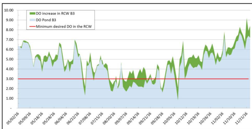
Fig. 4: Illustration of the early morning dissolved oxygen concentration in the pond (blue area) and inside the raceway (green area) in pond B3. The green area above the blue area indicates how much oxygen the aeration device added to the water at the entrance of the raceway, keeping dissolved oxygen levels inside the raceway often above 3 mg/L (minimum desired level) and seldom below 2 mg/L, even when pond DO approached values close to 1 mg/L.
