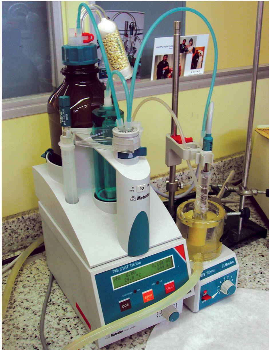
Hydrolysable protein is assessed in shrimp feeds and ingredients through a controlled reaction that simulates shrimp digestion.
