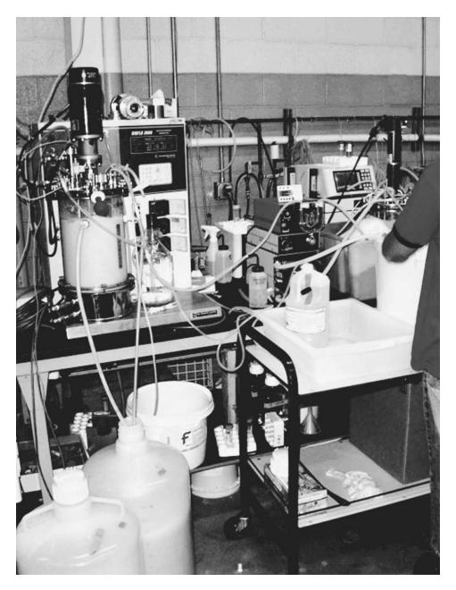
Separated soluble proteins and lipids are pumped to a second bioreactor for further pH adjustment to precipitate the muscle proteins.
