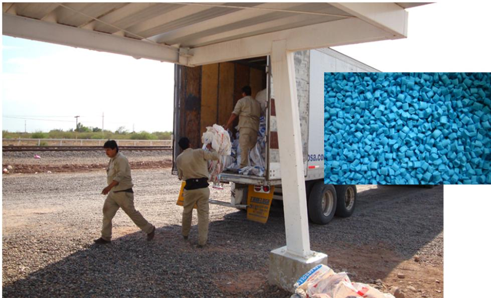
In the VIMIFOS program, thousands of feed bags are recycled and processed into plastic pellets used to make recycled plastic utensils.
