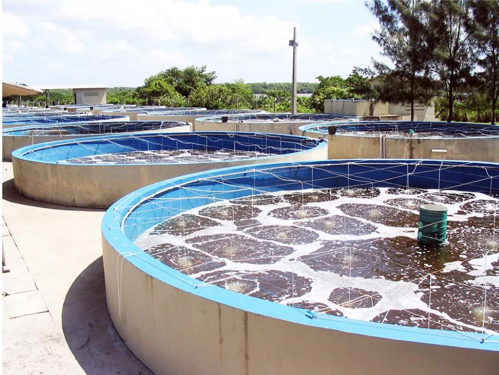
Diffused-air systems are most appropriate for smaller ponds and tanks with enough depth to allow oxygen to diffuse from the rising air bubbles into the water.
