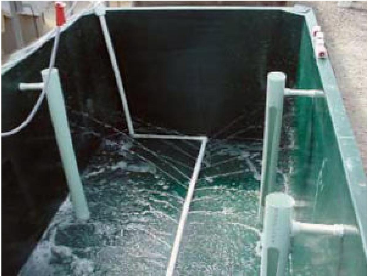
The tank design used a centerline for water distribution and airlift for water column circulation.
