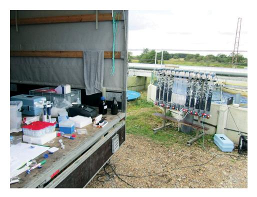
Easily degradable peroxyacetic acid residuals require immediate measurements, here with a simple mobile lab. The column set-up on the right is used to assess nitrification performance on biofilter elements exposed to disinfectant residuals.
