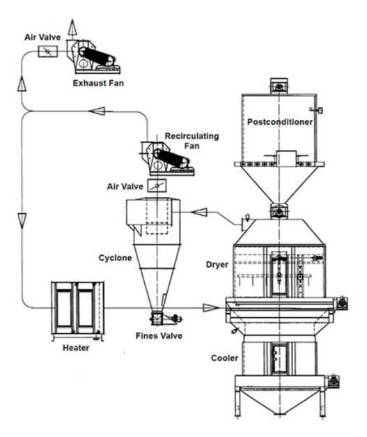
Postconditioner with drying and cooling package. Diagram courtesy of Geelen.
