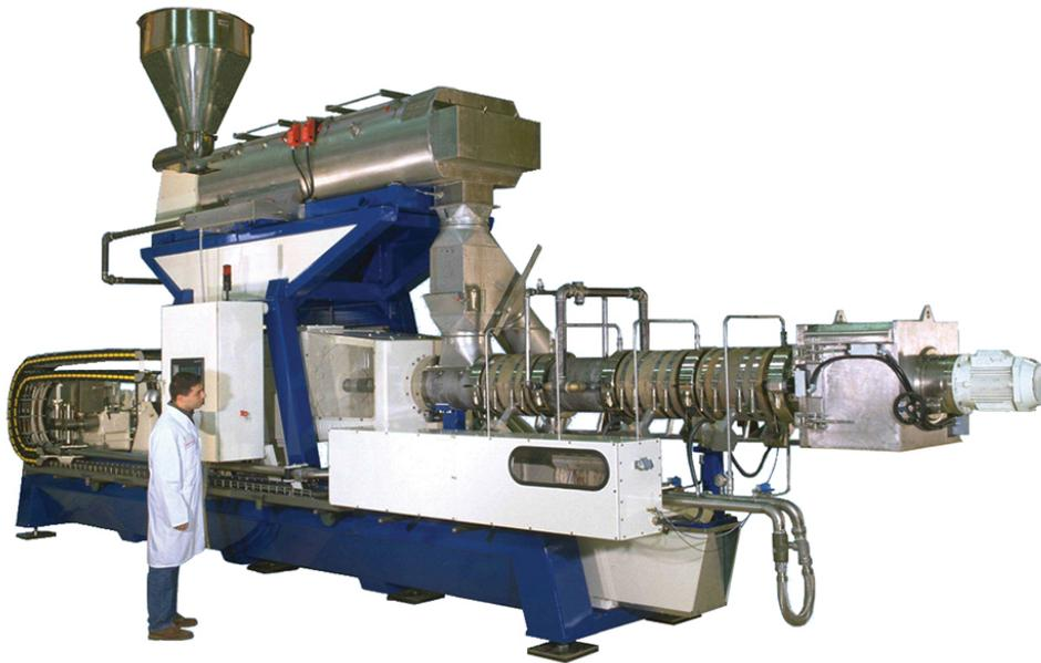
Advances in twin-screw extruder technology are quickly leading to greater control and flexibility in aquafeed manufacturing. Photo courtesy of Cletral Inc.
