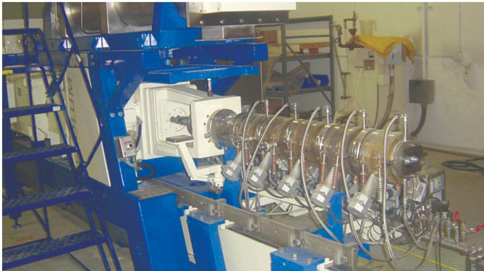
Simpler and less expensive than twin-screw designs, single-screw extruders offer a lesser range of functionality.
