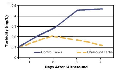
Fig. 1: Turbidity levels in catfish tanks.
