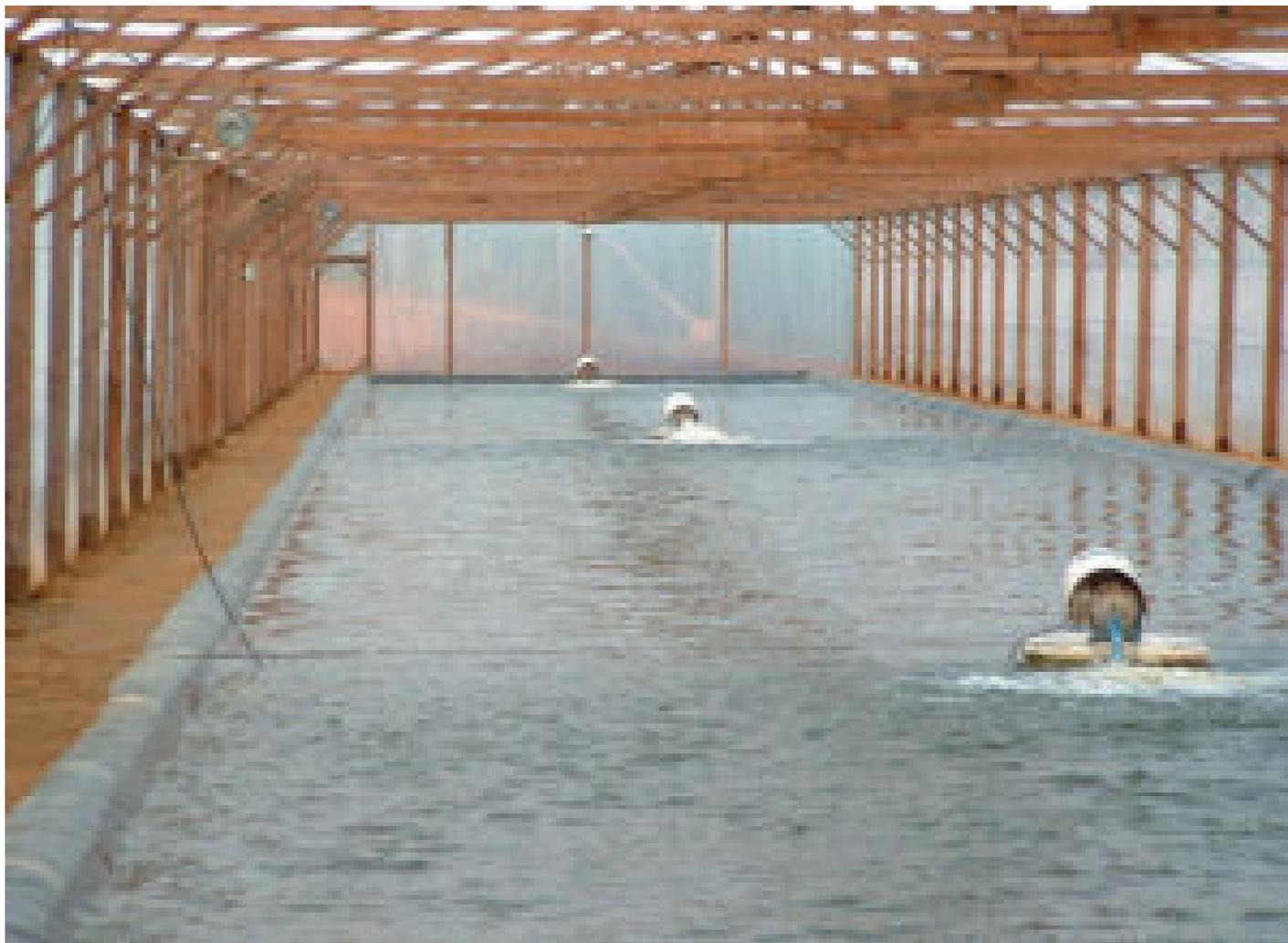
Propeller-aspirator pump aerators are very good mixing devices that are particularly useful for destratification.
