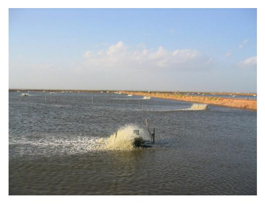
Proper mixing of water in aquaculture systems is important to distribute dissolved oxygen, fertilizers, liming and other products, and to prevent stratification of the water column. Photo by Darryl Jory.
