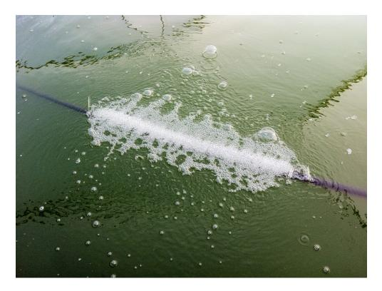
Diffuser hoses, typically placed on the bottom and supplied by air blowers, can be used to aerate the water column and provide mixing to aquaculture tanks and raceways. Photo by Darryl Jory.
