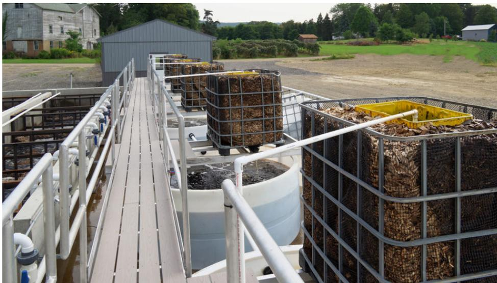
In TimberFish's novel RAS system, water is pumped across crates full of wood chips, sourced from nearby forests, which is studded with microbes. Photo by John Hand.
