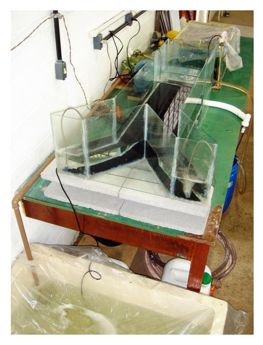
In each behavioral observation, two different ingredients were offered to shrimp at the same time, each in equal quantity at the end of each arm of the Y-maze test apparatus.
